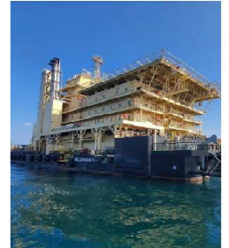
Millennium 3 Self-propelled DP2 Construction Support Barge
